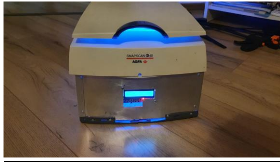
Ultraviolet lamp used to print the traces on the copper board
